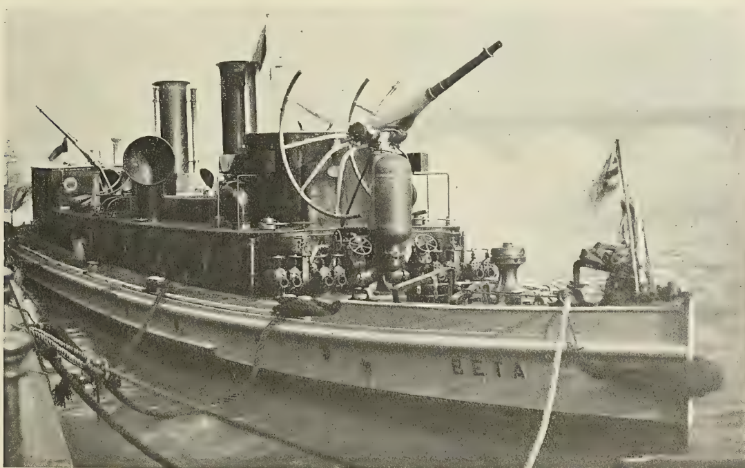
THE FIRE BOAT BETA, RECENTLY ADDED TO THE LONDON FIRE BRIGADE, SHOWING BIG MONITOR NOZZLE. (Copyright, Reginald Haines, London.)
